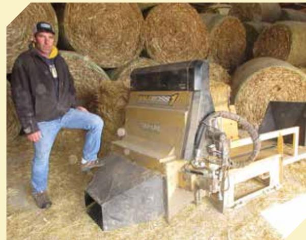
Rich modified a straw chopper mounted on a skid loader to blow fresh straw into each calf hutch.
